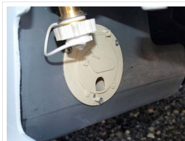
"Mousehole" with small opening for cord opened. The larger hinged plastic door opens to allow the plug through.
