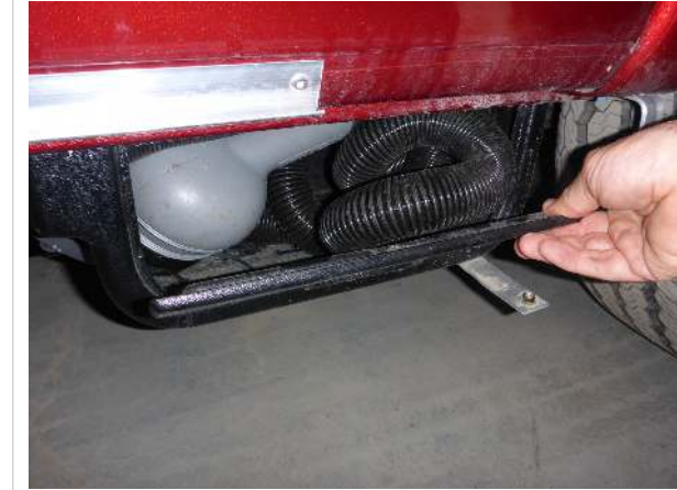
Waste water hose storage
