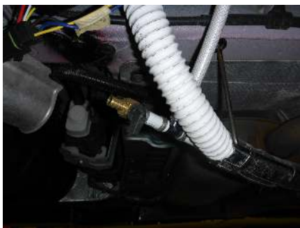
Fresh tank drain under the driver's door
