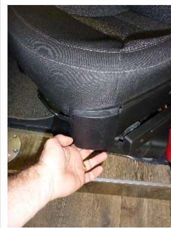
To rotate the front seats, lift up on the front inside corner trim
