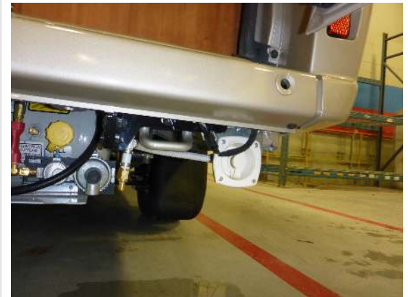
City water connection
