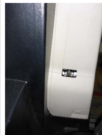
City water valve located in the B pillar on the driver's side (just behind the driver's seat)
