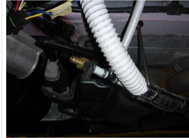
Tank drain, under driver's doorstep
