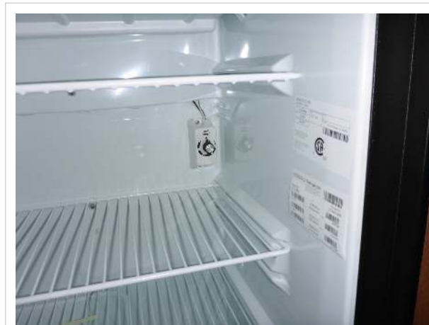
Thermostat is located inside on the rear wall
