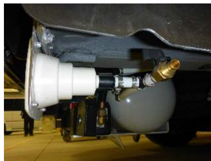
Drain by the fresh water fill in the rear
