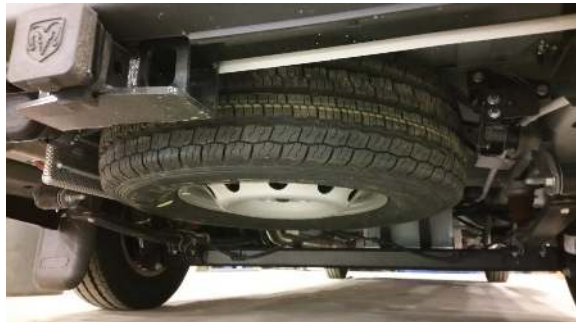
The spare tire is located behind the rear bumper
