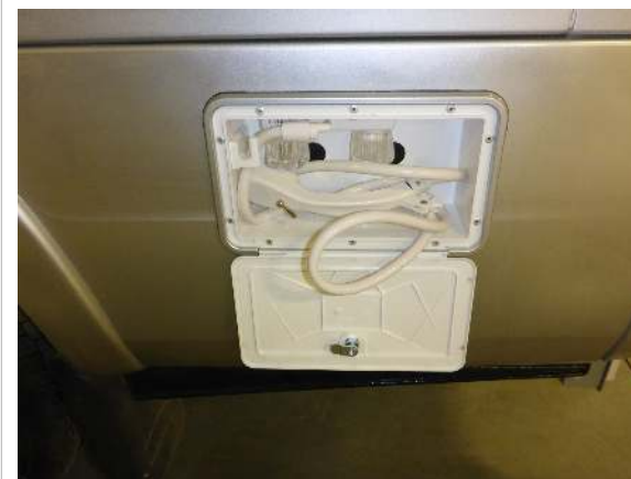
Rear compartment with outside shower faucet
