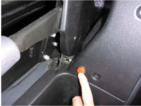
Macerator switch on driver's side doorstep
