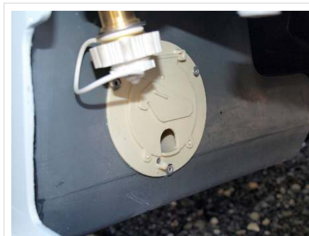
"Mousehole" with small opening for cord opened. The larger hinged plastic door opens to allow the plug through.
