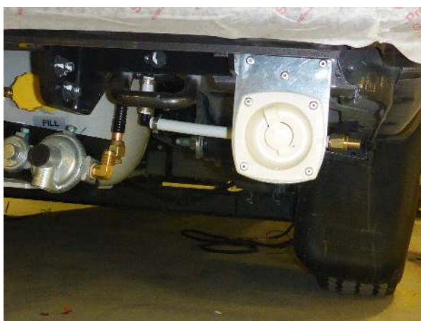
City water fill is on the passenger side, under the rear bumper
