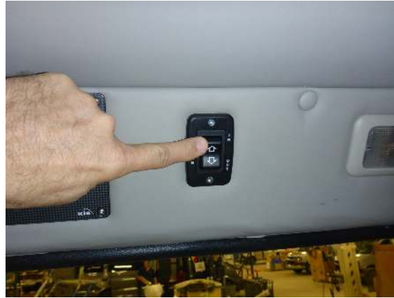
The awning power switch
