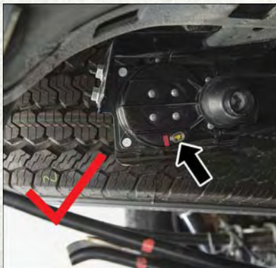
Winch Mechanism Properly Engaged (Yellow DOT Will Appear In The Winch Indication Window)
