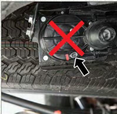
Winch Mechanism NOT Properly Engaged (Black Window Will Appear)
